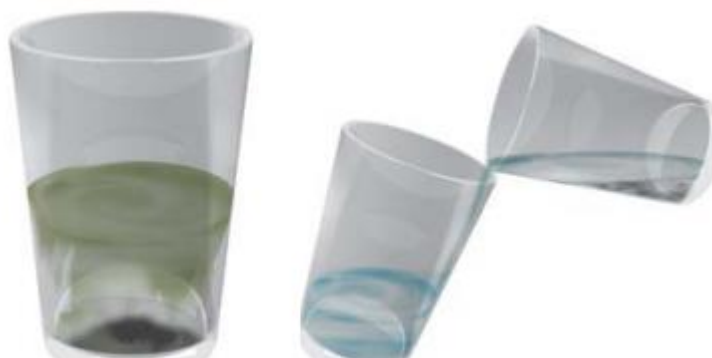
Figure 10: Sedimentation and decantation method:
