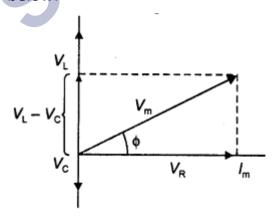
From the diagram, we observe that the vector sum of the voltage amplitudes  $V_R$ ,  $V_L$ , and  $V_C$  equals a phasor whose length is the maximum applied voltage  $V_m$ ,
