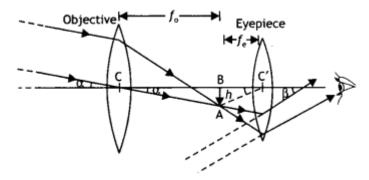
The object subtends an angle at the objective and would subtend essentially the same angle at the unaided eye. Also, since the observers' eye is placed just to the right of the focal point  $f'_2$ , the angle subtended at the eye by the final image is very nearly equal to the angle  $\beta$ .
