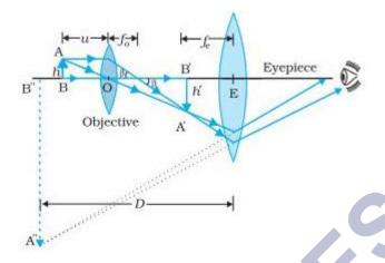
The first inverted image is thus near (at or within) the focal point of the eyepiece, at a distance appropriate for final image formation at infinity, or a little closer for image formation at the near point. Clearly, the final image is inverted with respect to the original object.
