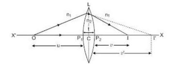
Let us consider the situation shown in figure.  $C_1$  and  $C_2$  are the centers of curvature of two spherical surfaces of the thin lens. O is the object and I' is the image due to first refraction. Let radii of curvature be  $R_1$  and  $R_2$ .
