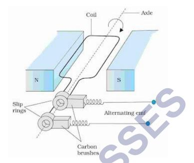
It consists of a coil mounted on a rotor shaft. The axis of rotation of the coil is perpendicular to the direction of the magnetic field. The coil (called armature) is mechanically rotated in the uniform magnetic field by some external means. The rotation of the coil causes the magnetic flux through it to change, so an emf is induced in the coil. The ends of the coil are connected to an external circuit by means of slip rings and brushes.
